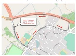
measured distance for calibration purposes. It will be marked with a yellow line on the road at the start and the finish. This is a loop of 1.65 miles. A mark will be on the road at exactly one mile, but here's a tip for easy calibration of Brantz, Terratrip and Monit machines. Zero the trip at the start and drive the route, ensuring not to cut corners and keep a regular distance from the kerb's edge. At the finish, make a note of the mileage shown on your tripmeter. Then use this calculation:
